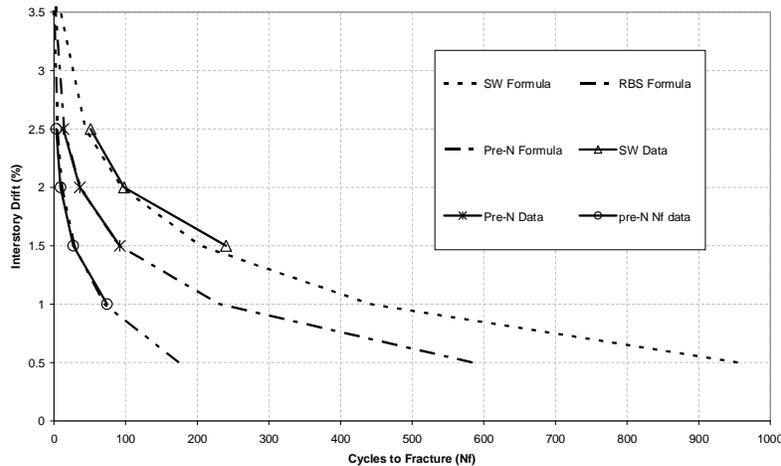
Figure 2. Sample fatigue life test data, W18x40 beams.
