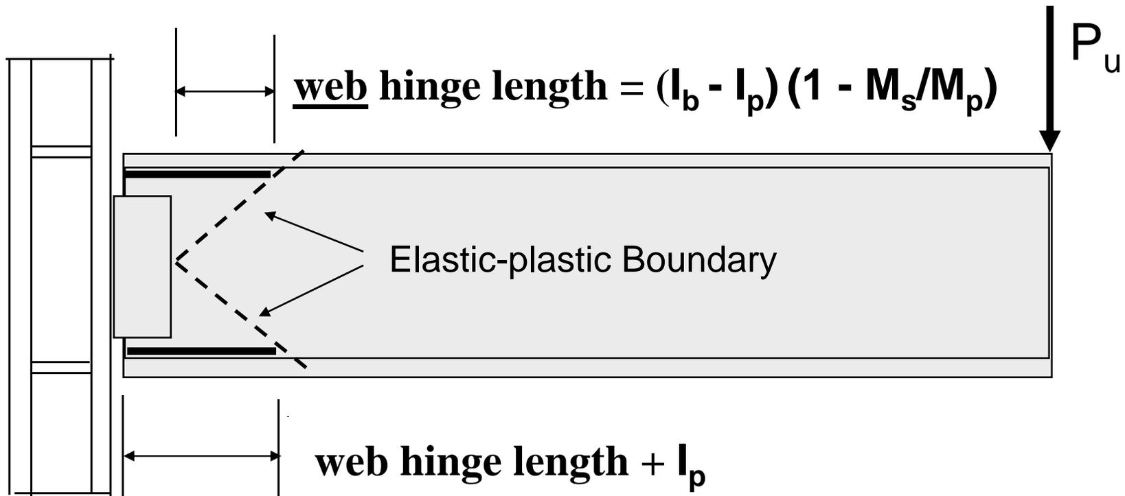
**The location of the centroid of the plastic hinge in the beam is located at the outboard edge of the shear plate.**
